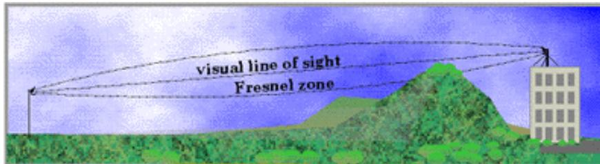
As shown in the picture above, when a hard object protrudes into the signal path within the Fresnel zone, knife-edge diffraction can deflect part of the signal and cause it to reach the receiving antenna slightly later than the direct signal. Since these deflected signals are out of phase with the direct signal, they can reduce its power or cancel it out altogether. If trees or other 'soft' objects protrude into the Fresnel zone,
