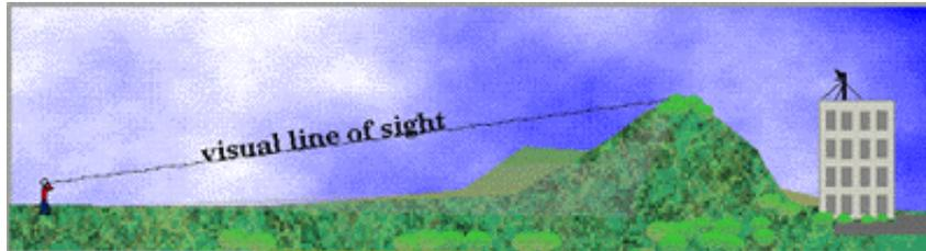
Obstructions that can interfere with visual line of sight can also interfere with radio line of sight . But one must also consider the Fresnel effect . If a hard object, such as a mountain ridge or building, is too close to the signal path, it can damage the radio signal or reduce its strength. This happens even though the obstacle does not obscure the direct, visual line of sight.
